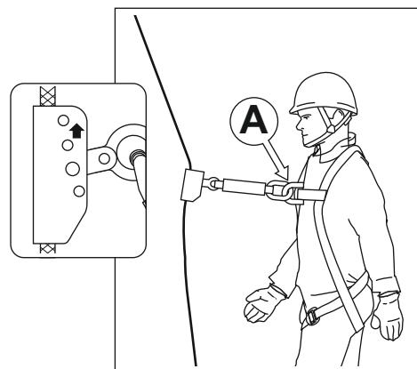
**ATTENTION:** Every time before using the equipment protecting against falls from height that employs the LINOSTOP II ED one needs to check if all the components are properly interconnected to one another and cooperate smoothly, as well as if they are compliant with compulsory standards:
